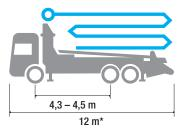
\*Dimensions varying according to truck assembly
