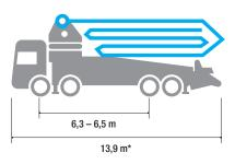
\*Dimensions varying according to truck assembly
